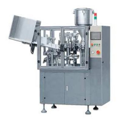
Fully automatic filling and sealing machine is a highly automated equipment for filling and sealing cylindrical metal hoses or composite hoses with paste materials. 316L stainless steel butterfly valve metering pump conforming to GMP standards, equipped with screw fine-tuning mechanism and accurate weighing. Adopting photoelectric marking mechanism, PLC programmable control, accurate and reliable trademark positioning.
