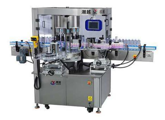
It can realize product positioning and labeling, using mechanical positioning, using the appearance and shape of the container itself to find positioning points, which improves the reliability of the equipment.
