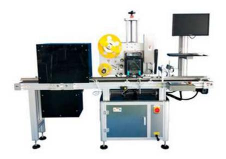
Visual And Code Reading Inspection Machine Series has vision camera inspection system, 300-200 million pixels, 16mm-100mm focal length lens, the camera uses software tools such as image comparison, average gray tool, banalization tool to detect and judge the third-phase information of the product, and the performance is reliable and stable.
