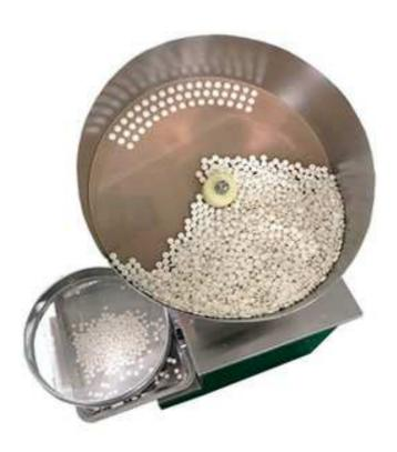
The capsule pill counting machine uses an electromagnetic vibration diameter. When the bottle does not turn to the blade, the bottle is not rotated. When the bottle is placed, the motor drives the number plate to rotate to automatically enter the bottle; replace different specifications model count Convenient and fast, there is no need to make other adjustments.
