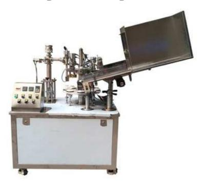
The automatic tube filling and sealing machine is suitable for various plastic tubes and aluminumplastic composite tubes for automatic color marking, filling, sealing, date printing and tail cutting. It is widely used in daily chemical, pharmaceutical and food industries.
