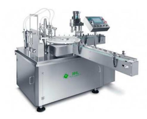
The series of products are suitable for filling of essential balm, medicated oil and other small bottle mouth products. The whole production process conforms to the new version GMP requirements. As the packaging materials are all irregular-shaped bottles, more robot functional devices or small machines are incorporated. It has various patented technologies with independent intellectual property rights. It has reached the advanced level and can substitute similar imported products.
