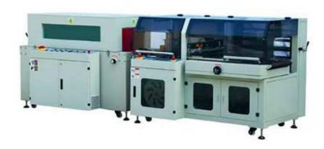
This machine has an imported PLC automatic program control, easy operation, safety protection and alarm function that effectively prevents incorrect packaging. It is equipped with an imported horizontal and vertical detection photoelectric, which makes it easy to switch selections. The machine can be connected directly with the production line, no need additional operators.
