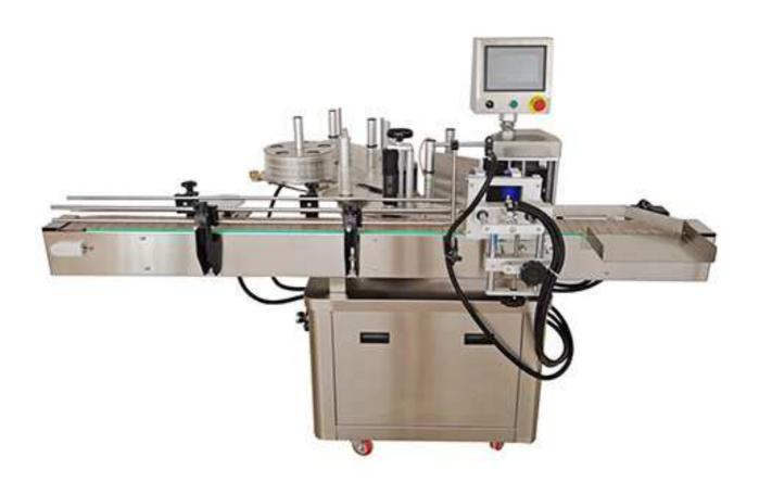
Automatic Labeling Machine can meet the needs of all round bottle labeling or semi circle labeling, bottle labeling switching between simple, convenient adjustment; Wide application range: self-adhesive labels, adhesive film, electronic monitoring code, bar code etc.
