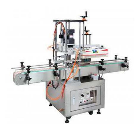
Side-wrap Capping Machine is used for all kinds of metal, glass and plastic bottles, which with the exceptions of crowns, ROPP (Roll-on Pilfer Proof) and straight wall corks style closures. It tightens screw caps from 20mm to 120mm in diameter, and it provides outstanding repeatable torque accuracy ensuring a high quality closure for every cap that it tightens. Designed to eliminate the strain of hand capping, it is a customer favorite for a very simple reason-it makes capping easy.
