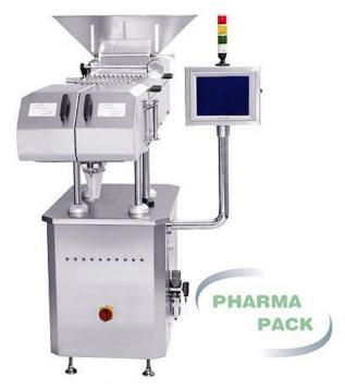
The counter PP-06 is a reliable, high performance machine, designed in conformance with current and proposed GMPs. Having a small footprint, they are effective in maintaining the integrity of a clean room environment. Few change parts are needed for different container sizes (only the nozzle). All product contact parts are made of type 316 stainless steel. And all contact parts can be easily disassembled for cleaning.
