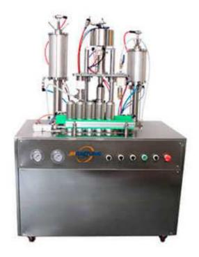
1600AT aerosol machine is a new design automatic aerosol filling on the basis of 1600A. It consist of liquid filler, valver inserter, sealing machine, gas filler. Use the screw bottles pusher instead manual work. It has two working model: manually intermittent filling and automatic intermittent filling. Intermittent time is adjustable, very flexible and efficient.
