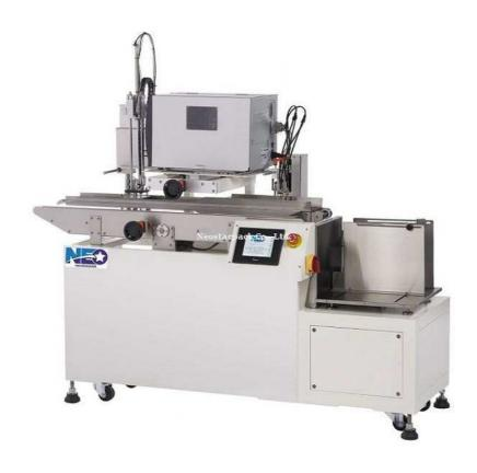
NLS-450PB Print and apply labeler with feeder can apply preprinted labels on bags fed automatically by bag feeder. The application include identification and tracking, (RFID) tags, and variable information (weight, ingredient, etc) Cards or other material or sizes of bags is also available to be applied on this print and apply labeler with feeder.
