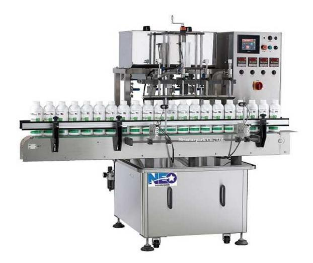
NFP-460 suits for various low viscosity liquid, such as lotion, syrup, cleanser, etc. No adjustment is required as changing products and discharge vast volume to achieve high productivity with excellent accuracy.
