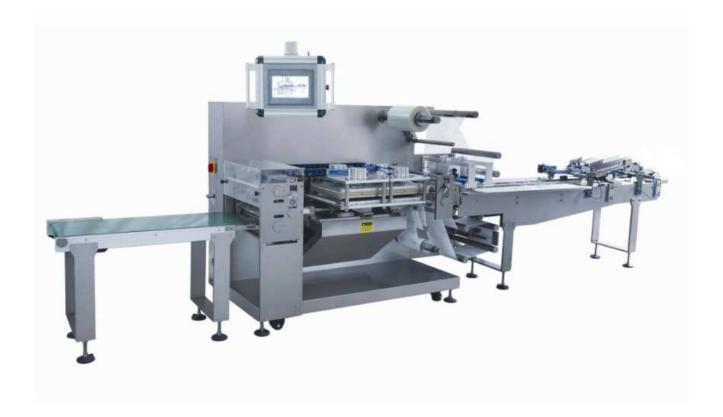
**YSB-380** fully automatic medical four side seal packing machine is specialized for the domestic and foreign medical packing industry, It is developed for automatic package industry of flat material such as dressing, indwelling needle, surgical sewing kit, plaster gauze sheet material and so on. This machine gathered mechanism, electricity and gas in one, derived by four servo motor, and equipped automatic feeder, adopted the PLC program controller, making the machine running procedures.
