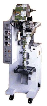
It has been developed latest according to international fashionable style. The appearance of bea is very smart and packaging material is used efficiently. The machine adopts the structure of horizontal sealing and cutting as one and no damage bags appear. Model DXDK60 II is suitable for packaging grain; Model DXDP60 II is suitable for packaging tablet; Model DXDL60 II is suitable for packaging liquid; Model DXDF60 II is suitable for packaging powder.
