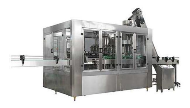
The BRGF series filling machine mainly used in glass bottle packing.
