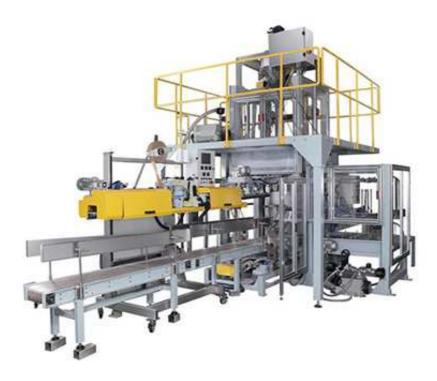
Our company is a new type of packaging unit for powder material packaging in agrochemical and food industries. The unit has automatic bag feeding, bag loading, filling, bag feeding, sealing and other functions. Can work with all kinds of powder material equipment linkage, to achieve large size packaging unmanned production operations.
