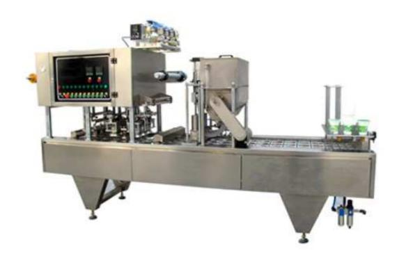
Automatic cup filling and sealing machine is applicable for liquid, semi-liquid, powder and granule filling into cups, bowls and plastic boxes etc. The filling containers can be round, square and special shaped in plastic (PS, PP, PVC, PET, etc) and paper (there should be a film inside the surface of container). This machine is widely used in beverage and food industries.
