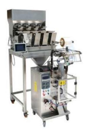
This packing machine is for granule, dry & loose powder, nut, in chemical industry, pharmacy and foodstuff industry
