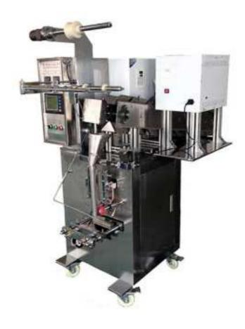
This is a stainless steel made vertical packing machine which is mainly used to pack tea, small granule material.
