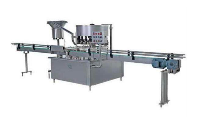
This machine is intended for capping bottles of infusion solutions. The equipment comes with a high-power generator of electromagnetic waves for complete set caps, which reduces the labor intensity. In addition, the device provides high performance by smooth and continuous operation of bottles available.
