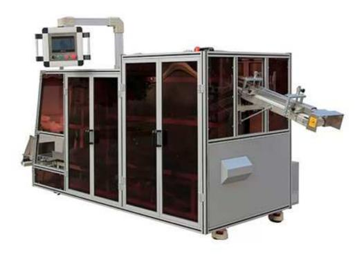
Automatic flat pocket bagging machine for packaged noodles
