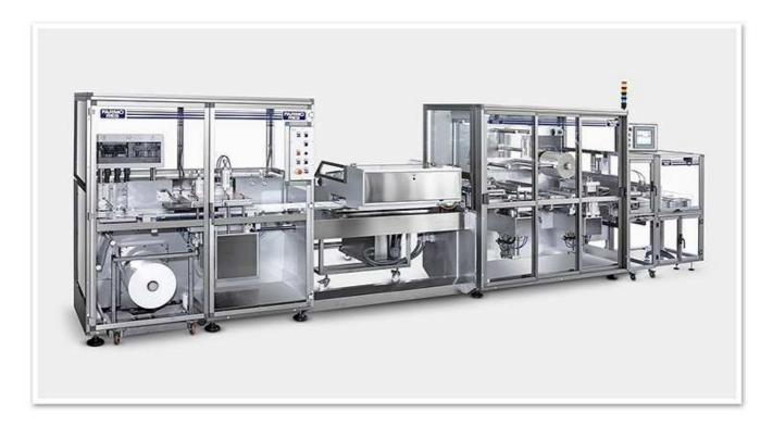
The KB models are the new automatic thermoforming machines with a balcony constructed frame and pneumatic actuating systems for packing syringes vials and ampoules in laminated plastic materials. Technical innovations: compact frame, automatic positioning of sealing, perforation and cutting station, operator side reel loading, improved design so using less space in the loading area.
