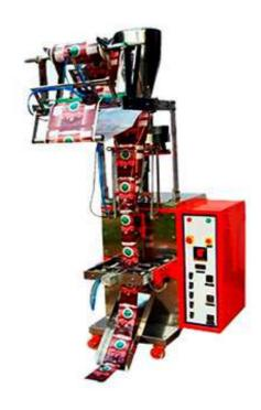
We manufacture and export Form filling and sealing machines. This machine is used for packing of powder and free flowing products. Automatic pouch packing machine (Chute type) fitted with volumetric cup filling system is used to pack only dry granular and free flowing powder items such as Rice, Tea, Pulses, Detergents, Seeds, Cereals, Sugar, Salt, Glass Beads etc.
