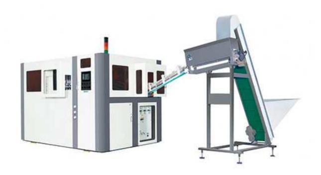
Energy-saving type plastic Bottle Blowing Machine is suitable for mineral water, medicine, oil, alcohol, carbonated drink, cosmetics, high temperature resistant bottles and so on.
