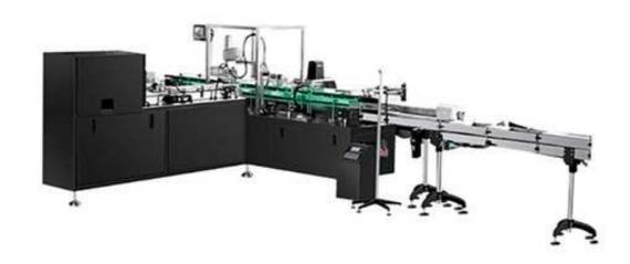
The AFPAK AF-B10 is specially designed to pack K cups into box solutions.
