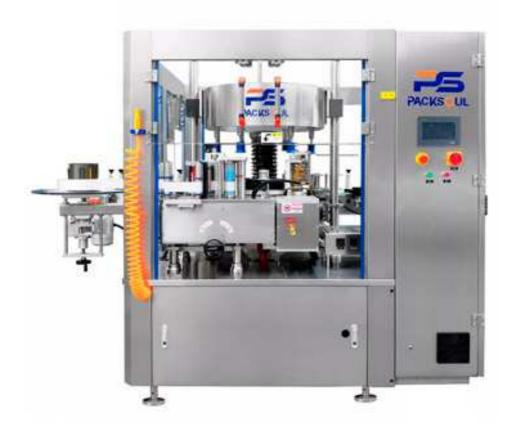
PSR-640 rotary type opp labeling machine is design for big bottle, big bucket or other large volume container whether empty or filled, which can satisfy the labeling requirement of 5-15L, 5 gallon, or large volume product and so on. In addition, PSR-640 also suitable for various shape such as round, rectangle, square etc.
