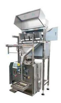
Automatic packaging machine is a kind of automatic packaging equipment, which is upgraded on the basis of particle packing machine. It can automatically complete all the work such as the measurement, bag-making, filling, sealing, printing batch, cutting and counting and so on, automatically complete the packing of the fine particle-like substance. The electrical-sensor detects the color marks on the packing film to keep a perfect picture on each bag.
