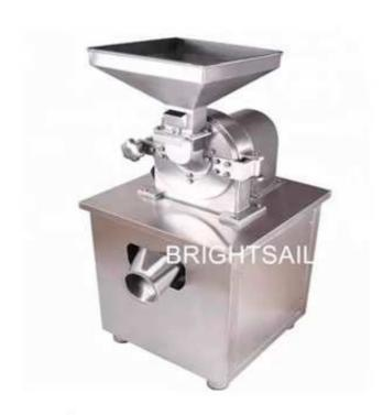
BSU universal crusher is suitable for grinding spices, crystal materials, grain and so on. It usually has 3 types knives for your choices, hammer type, turbo type, pinned disc type. We will recommend you the suitable knife type according to your raw material and particle size.
