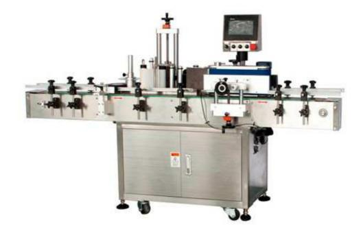
DLTB-A Round bottle labeling machine is economical, self contained, easy to operate, equipped with auto teach programming touch screen. Built in microchip storing different job setting makes fast and easy changeover. This automatic labeling system is ideal for cylindrical container.
