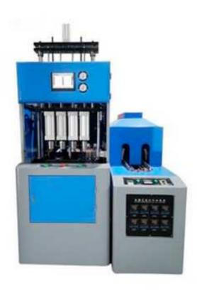
Semi automatic bottle blow molding machine is suitable for producing PET plastic containers and bottles from 0.1L to 20L. It is widely used to produce the mineral water bottle, carbonated drink bottle, Juice bottle, pesticide bottle, oil bottle, daily chemical bottle, cosmetics bottle, wide-mouth Jar, PET can etc.
