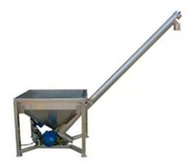
ZH-CS2 screw conveyor is developed for conveying powder product, such as milk powder, rice powder, sugar, gourmet powder, amylaceum powder, washing powder, spices, etc.
