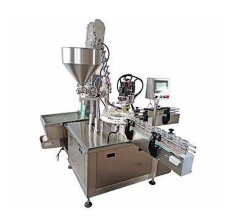
This automatic production line is designed with multiple function, it can arrange bottles, fill liquid or paste, feed bottle plugs and caps, cap bottles and sort finished products automatically. It can help you improve working efficiency. This is suitable for essential oil, water, juice etc. We can customize the machine and make it can work for different sizes of containers at the same time.
