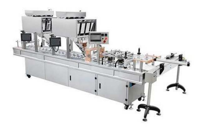
Granular Cup Filling and Sealing Machine is suitable for automatic filling of granular materials in food, pharmaceutical, chemical, pesticide and other products. Such as: nuts, peanuts, melon seeds, potato chips, peanuts, oatmeal, penghua food, desiccant, broken tea, granules, coffee sugar, white sugar and various non-sticky loose particles, etc.
