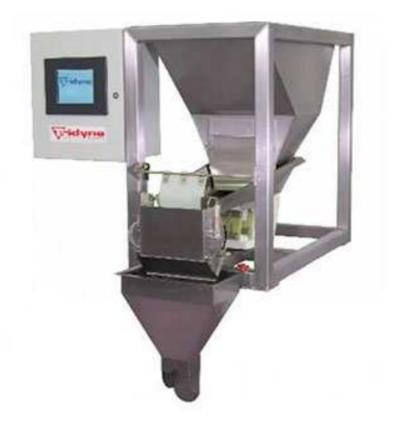
The Tridyne F-100 Series of Net Weigh Fillers are available in 4 different configurations. It can be used as a table top model or can be integrated with other industrial bulk filling equipment such as baggers, conveyors, sealers and more. Products need to be free flowing.
