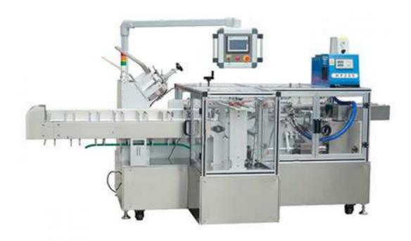
The cartoner Machine automatically picks the carton and forms the carton, worker manually puts the products on the moving conveyor, and when it's moving to the formed carton, the machine pushes it into the carton, sealing the carton with glue. If you want to save the labor cost, you can add a robot to place the goods on a conveyor instead of one person.
