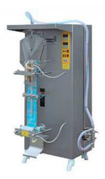
SJ-1000 Liquid packing machine widely used to pack milk, soybean milk, sauce, vinegar, yellow wine, all kind of drink with film. The whole process can be accomplished automatically, such as ultraviolet sterilization, bag figuration, date printing, quantitative filling, enveloping, cutting, counting, and so on. The temperature of heat-sealing is controlled automatically, the production is beauty and fastness, the machine adopts stainless steel shell, and the sanitation is guaranteed.
