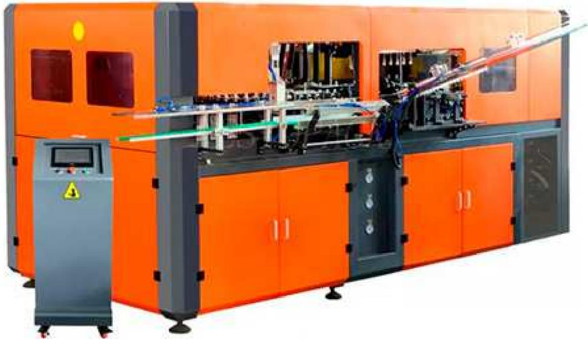
Automatic PET bottle blow moulding machine is suitable for blowing plastic containers and plastic bottles of any shape with pet as the main raw material. It is widely used in blowing carbonated beverage bottles, mineral water bottles, oil bottles, pesticide bottles, cosmetic bottles, etc.
