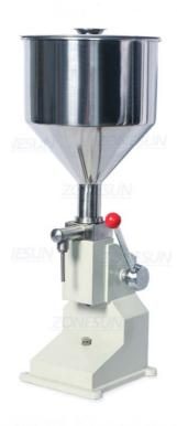
The manual filling machine is specially designed by our factory for medium or small size enterprises, laboratory, hospital or beauty parlor in daily use chemical section. Its cofiguration is compact, acts agility and easy to use, all the parts which dip in the material are made of stainless steel.
