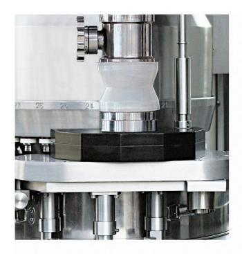
The force feeder device could improve liquidity and filling for the pellet.
