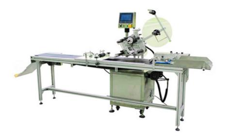
This labeler is designed for labeling on flat sides of thin and soft products.
