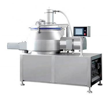
The machine is a process machine widely applied for solid preparation production in the pharmaceutical industry. It has such functions as mixing, granulating, etc. It is widely used in such industries as medicine, chemical industry, food, etc.
