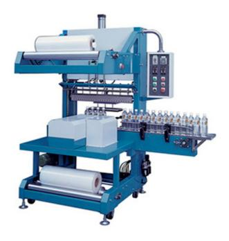
A CHM-6030CF sleeve wrapper is used to seal the important commodities like packing of beer, beverage, mineral water etc. without a tray and it is also known as counting & forming sealer. To get the wrapping and shrink solution this machine can be combined with shrink packaging machine. PE and PVC film is used for packing of various commodities.
