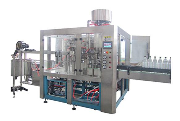
PCGF24/24/8 Beer Rinser-Filler-Capper Monobloc is an high efficient automatic liquid packing machine, which perfectly combine bottle rinsing machine, pressure filling machine and capping machine together in one unit.
