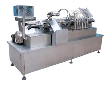
The machine is a new generation of the ampoule drawing, filling and sealing combined equipment for injections. It adopts the rectangular feeding instead of the traditional ampoule feeding methods. In such case, the feeding is steady with no easy broken ampoule.
