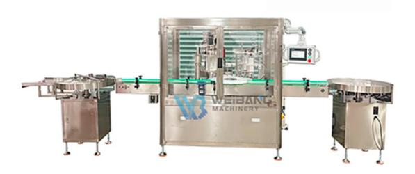
Powder bottle filling machine is one kind application of auger filler or auger dosing machine. It is suitable to fill 5 grams to 5000 grams of any powder in rigid containers including plastic bottles, glass bottles, metal tin cans, jars, tubs, buckets, boxes, drums and pails.
