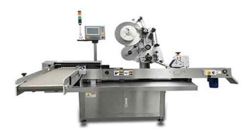
Process: horizontal feeding  $\rightarrow$  screw splitting  $\rightarrow$  batch printing  $\rightarrow$  horizontal labeling  $\rightarrow$  defective product detection and rejection  $\rightarrow$  finished product  $\rightarrow$  next process
