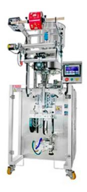
This type of small vertical packaging machine is an upgraded model of CB-280, with optional reciprocating sealing jaws, special shape bag packaging, and multi-material combinations.
