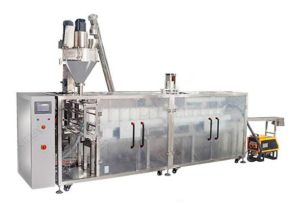
The flour paper bag packaging machine has been designed with the objective of reducing production costs for high-volume use, but at the same time, offering a high degree of versatility for smaller fill weights of up to 2 kg.
