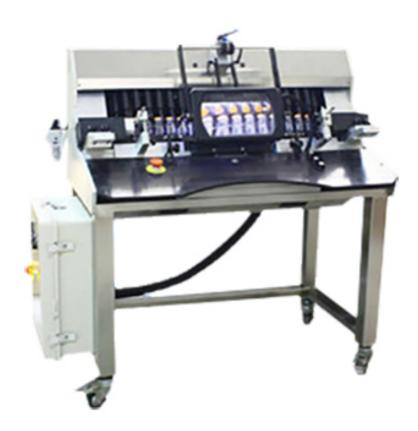
Inspection Machine Model YJ-350 is mainly used to inspect pharmaceutical preparations in bottles such as vials.
